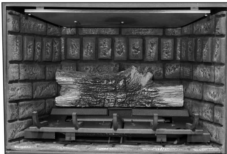
Figure 53: Install the back log on top of the pilot on the back shelf of the air deflector. Push it against the back brick panel.
