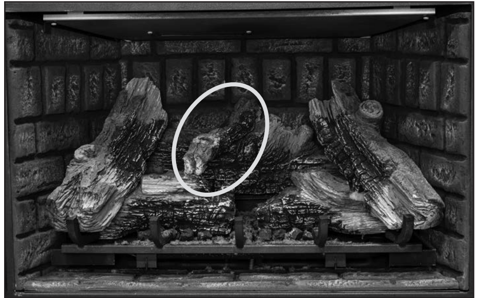
Figure 58: Place the center top crossover log at an angle on top of the rear log and left mid log pins
