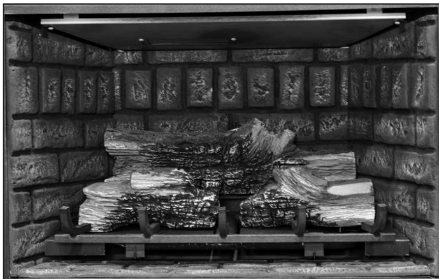
Figure 54: Place both the left and right mid logs in the middle of the air deflector. Make sure the bottom holes align with the pins in the air deflector.
